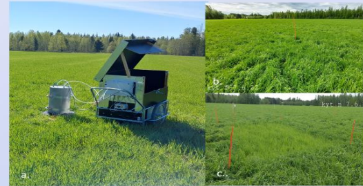
Fig. 3: a. Gas measurement system (chamber and cart with analysers), b. measured grassland and c. non-fertilized plot measurement plot
